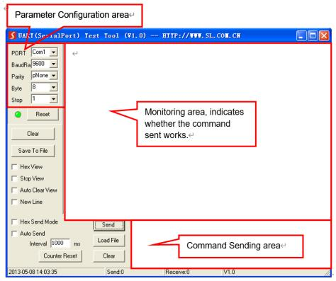
Please set the parameters of COM number, bound rate, data bit, stop bit and the parity bit correctly, only then will you be able to send command in Command Sending Area.
